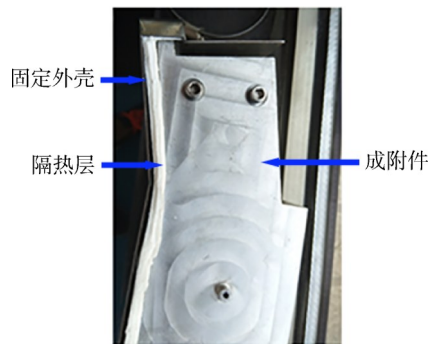
图 6 附件硅酸铝隔热层加装示意图 Fig.6 Sketch of the installation of aluminum silicate of the accessories
